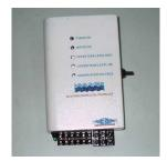
Once Hydrokon is attached to your pump-motor, the pump-motor automatically starts when the water level drops below a certain level. When the water level reaches a certain level, Hydrokon automatically stops pumpmotor. These levels are determined by the user.
